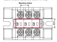
• When using the marking strip, calculate the length as shown in the "Dimension calculation" table on the right.
