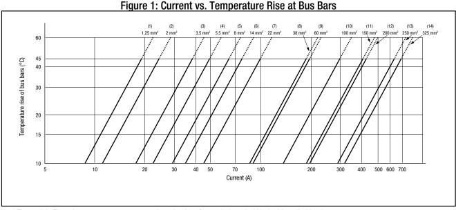
Note) The graph in Fig. 1 shows current vs. temperature rise at bus bars for a typical terminal block with applicable wires. Test conditions are in accordance with JIS C 8201-7-1.
