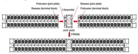
• Use the below screws when installing the joint plate.
